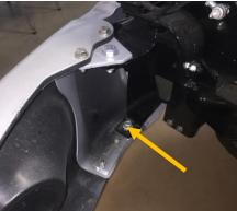
3. Using <sup>3</sup>/<sub>4</sub>" wrench and socket, remove the nut on the top bolt attaching bumper to frame. (both sides) Close hood and remove bumper. Set bumper aside.
