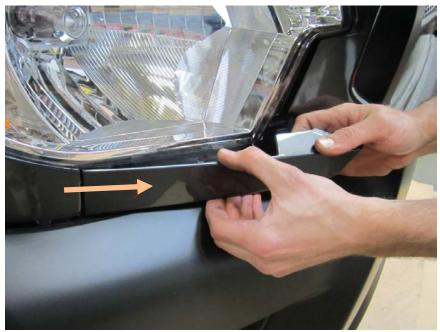
10. Remove OEM bumper cover by gently pulling away from the truck. (both sides)
