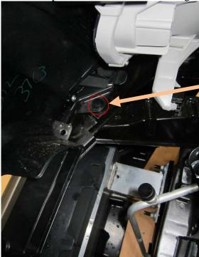
5. Using flathead screwdriver, remove plastic quarter turn fastener. Then, using 10mm socket, remove screw in fender well. (both sides)
