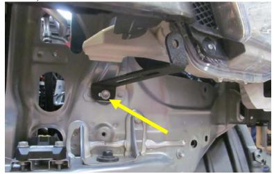
4. Reinstall OEM headlight trim by pressing clip through the hole in the Hammerhead headlight trim tab. (both sides)
