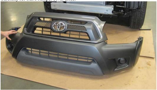
12. Remove 8 tabs on bottom inside of grille to separate OEM bumper cover from grille.
