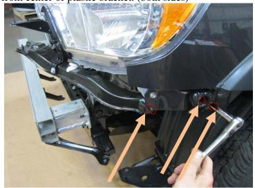
15. Remove side OEM support structure and set aside. This will not be reused. (both sides)
