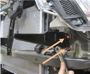
18. Using 14mm socket, remove six nuts from aluminum OEM bumper. Pull away from truck to remove.
