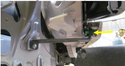
5. Using weldnut tabs provided and hardware kit #64, install and align hammerhead bumper. Ensure that each ½" bolt receives a flat washer and lock washer.
