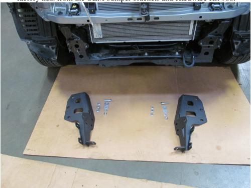
2. Slide frame mounts over factory bolts and install OEM nuts. Install a ½" bolt, lock washer, two flat washers, and a ½" nut in the bottom tab of each frame mount. Hand tighten ONLY.
