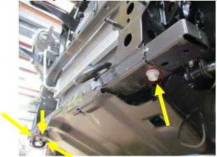
21. Remove frame rail ends by pulling away from center of truck. These will not be reused.
