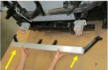
19. Using 14mm socket, remove three nuts from aluminum OEM bumper bracket. (both sides)
