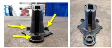
7. Using the Torx 20 socket, install the OE bolt plate and camera mount onto the Spare tire Adapter using the two OE screws as shown below.
