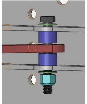
5. Using a 9/16: socket, install the 3<sup>rd</sup> brake light bracket and the Spare Tire Adapter onto the Spare Tire Carrier as shown. Use the 4 carriage head bolts, washers, and nylock nuts from hardware kit #152. The brake light bracket and spare tire adapter are adjustable vertically for different size tires. (35" in the lowest position, 40" in the highest position.) IT IS VERY IMPORTANT TO TIGHTEN THESE BOLTS TO SPEC OR RISK HAVING YOUR SPARE TIRE FALL OFF THE VEHICLE
