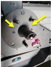
8. Route the Camera and 3<sup>rd</sup> brake light wires through the hole shown below.
