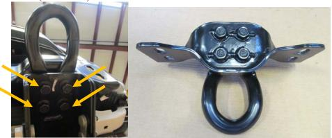
5. Using 18mm socket, remove two nuts attaching underrun bracket to frame. Set aside; it will not be reused. (both sides) Bolt strips and nuts will be reused.
