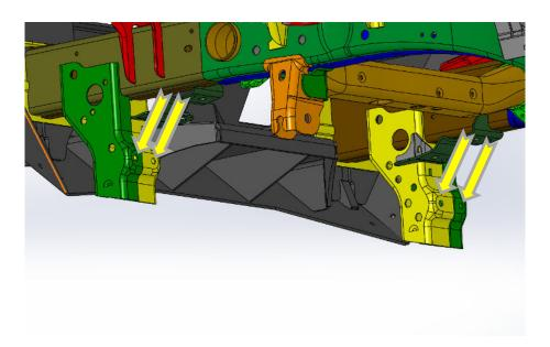
2. Using a 9/16" socket, mount the Front Skid Plate with the provided 3/8" nuts and washers.
