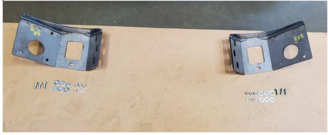
7. Attach frame mounts to frame as shown. Do not fully tighten.
