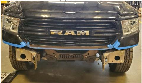
8. Using a hoist or a few friends, attach bumper to frame mounts using hardware kit #58 and weldnut tabs. Start all bolts before aligning bumper. Leave a minimum of 3/8" space between bumper and truck body. When the truck flexes off-road, this distance allows your bumper and truck body to have clearance. Tighten bolts with <sup>3</sup>/<sub>4</sub>" socket and wrench. Tighten frame mount bolts at this time.
