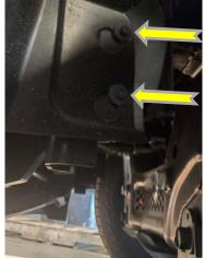
3. Unplug automatic spoiler located under bumper. Using a 13mm socket, remove four nuts attaching it to frame. Set assembly aside, it will not be reused.
