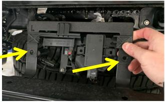
10. Using a 21mm socket or wrench, remove lower tow hitch bolt and place frame mount in position as pictured below. Note – notch goes up for 2500 & 3500 models, notch goes down for 1500 model. (Passenger side). Do not fully tighten.
