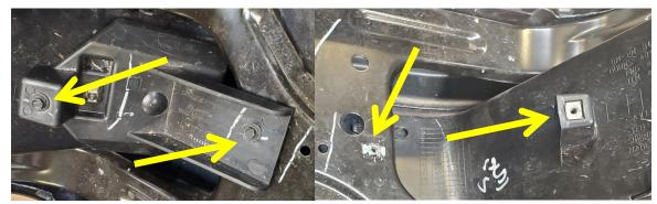
2. Install sensor and senor clips into bumper carefully. Be sure to orientate all sensors in the same direction as the OE bumper.
