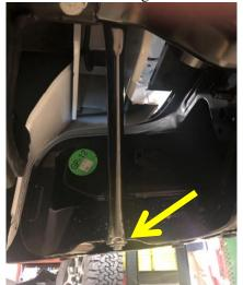
4. Using 18mm socket or wrench, remove two nuts attaching OE bumper to receiver hitch. (both sides)
