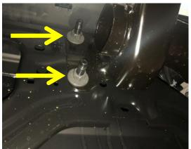
5. Using trim tool, remove one plastic retainer attaching wire loom to bumper. (arrow) Leave module plugged in. Unclip module out of bumper and allow it to hang down.
