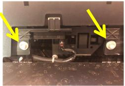
7. Using 21mm socket, remove nut attaching side brace to frame. Remove brace and replace nut.
