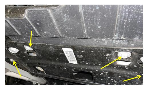
6. Gently remove the bumper from each side of the vehicle where the bumper and fender meet. To do so, pry the fender flair outwards detaching it from the bumper cover. Release the clips behind the bumper by gently pulling outwards. As doing so, work your way to the center of the bumper. Repeat for other side.
