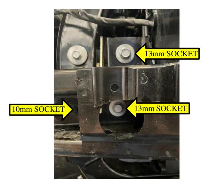
9. Using a 13 mm socket, remove the two hex head (1 per side) bolts holding the crash bar support to the cross member. Set hardware aside to be reused.
