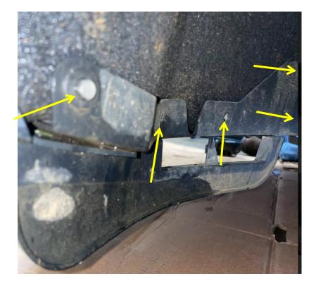
4. Looking at the engine splash cover on the bottom of the bumper, use a 10 mm socket to remove the three hex head bolts located in the indentions. Set hardware aside to be reused.
