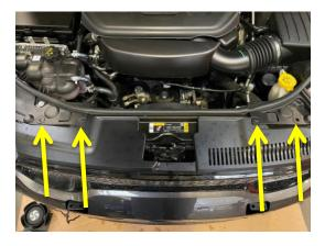
2. On each side of the vehicle locate the 4 plastic rivets (2 per side). Using a trim removal tool pry the head and body of the rivets out. Set plastic rivets aside to be reused.
