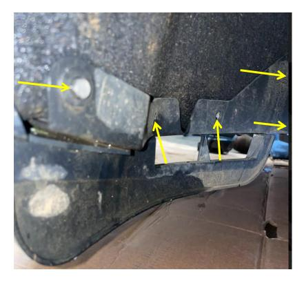
11. Using 4 plastic rivets, re-install the grille shroud by pushing the rivets in the holes located by the arrows in the picture below.
