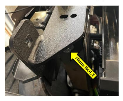
3. Using a 13mm socket, install the crash bar support over the right frame mount weldment using OE hardware. Repeat for other side.
