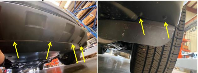
9. Using a 7mm socket, locate the 8 flange bolts (4 per side) at the bottom of the fender liner. Reinstall the bolts to the side bumper from the fender liner.
