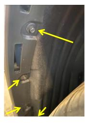
4. On the bottom of the bumper, located the 5 flange bolts in the center and 2 flange bolts in front of each wheel. Use a 7 mm wrench or socket to remove the nine flange bolts. Set hardware aside to be reused.
