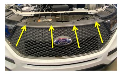
2. On each side of the vehicle, locate the 6 plastic rivets (3 per side). Using a trim removal tool pry the head and body of the rivets out. Set plastic rivets aside to be reused.
