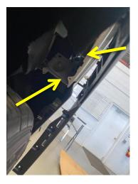
10. Using a 7mm wrench or socket re-install the 5 flange bolts on the bottom of the bumper in the center and 2 flange bolts in front of each wheel.
