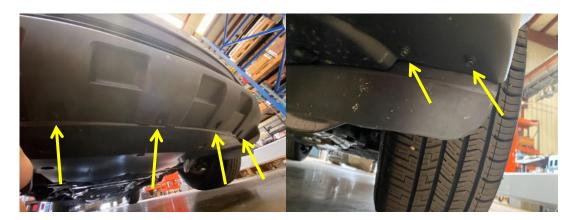
5. In the wheel well pull back the liner and locate 4 flange bolts (2 per side). Using a 10mm wrench or socket remove the 4 flange bolts. Set hardware aside to be reused.
