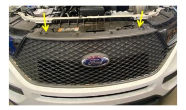
7. With the bumper removed, you can now remove the upper and lower air inlets.
