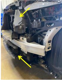
8. Using a 13 mm socket, remove 8 hex head bolts (4 per side) from the bumper bar as shown below. Do not remove the bumper bar. Set hardware aside to be reused.
