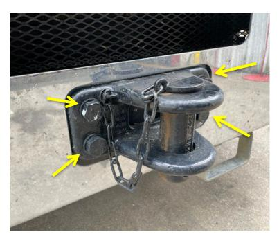
2. Using a 19mm socket or wrench, remove six bolts attaching OE bumper to frame of truck. Using a crane or hoist, hold weight of bumper while removing bolts. Remove bumper and set aside.
