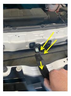
4. On the bottom of the bumper, located the (6) M7 bolts in the center and (4) T15 screws on each side in front of the wheels. Use a 7 mm wrench or socket to remove the (6) M7 bolts and a T15 to remove the screws in front of each wheel. Set hardware aside to be reused.
