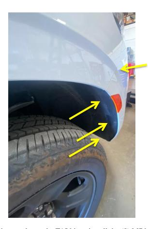
8. Using a 7mm wrench or socket and a T15 bit re-install the (8) M7 bolts and (6) T15 screws in the bottom of the bumper. Note: Start in the center of the bumper and work out towards the wheels.
