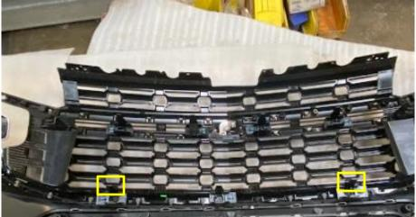
6. Now the slots are complete, use a hoist or a friend to lift bumper to be snapped back on. Align the bumper slots to the push bumper mounts and slide the bumper on. Start attaching the bumper from the center and working your way out. This allows for the clips to line back up properly making sure the bumper is on correctly. Work your way out to the fender flairs.
