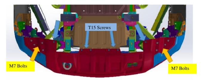
5. Next with a 10mm socket or wrench begin by removing the (6) 10mm bolts holding the top of the grille to the radiator support. With the bolts removed, remove the bumper by lifting up the top of the grille. There are two clips holding the bumper in place, lifting up and pulling forward on the bumper to remove it from the vehicle. Remember to unplug any wiring harness.
