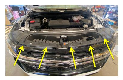
2. On each side of the vehicle, locate the (6) T15 screws (3 per side). This will give you access to the (6) 7mm bolts (3 per side) holding the fender onto the body. Remove these and set aside for reuse.
