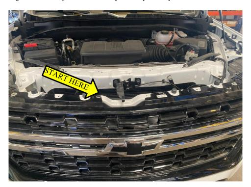
7. Using a 7mm wrench or socket reinstall the (6) flange bolts (3 per side) from the fender wheel well to the bumper. Followed by installing the (6) T15 (3 per side) screws in the inner fenders as well.
