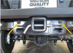
4. Remove trailer connector, sensors, sensor grommets, spare tire access lock, and wiring harnesses from bumper.
