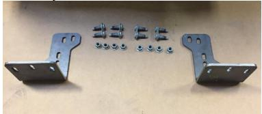
8. Install Hammerhead frame mounts on frame as shown using OE bolt strips. Slide mounts away from truck as far as possible. Do not fully tighten.
