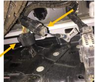
2. Using 21mm deep well socket, remove four nuts attaching bumper to frame. (both sides)
