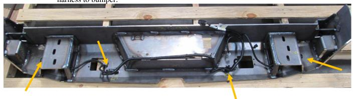
5. Install accent plates: Start by applying the foam weather stripping included in the install kit to the edges of each accent plate as shown in the picture below. This prevents rubbing between the accent plates and the bumper.
