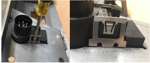
3. Install OE sensor grommets and sensors in bumper.
