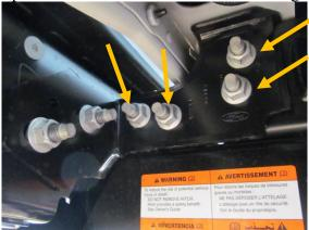
3. Using 13mm socket, remove two bolts attaching bumper to receiver hitch. Bumper is now ready to be removed. Set aside; it will not be reused.
