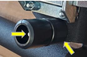
4. Install bumper mount brackets to the brush guard with (2) shoulder bolts, (4) spring washers, (2) flat washers, and (2) hex nuts from hardware kit #203. Use shim #1 between the shoulder bolt and hinge. Place a spring washer between the hinge and bumper mount. Tighten with a 9/16" wrench and ¼ Allen key.
