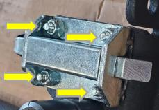
3. Install rubber compression springs with (2) 7/16" hex bolts, (2) flat washers, and (2) nylock nuts from hardware kit #203. Place shim #2 between compression spring and brush guard. Tighten with a 7/16" socket and T-30 torx.
