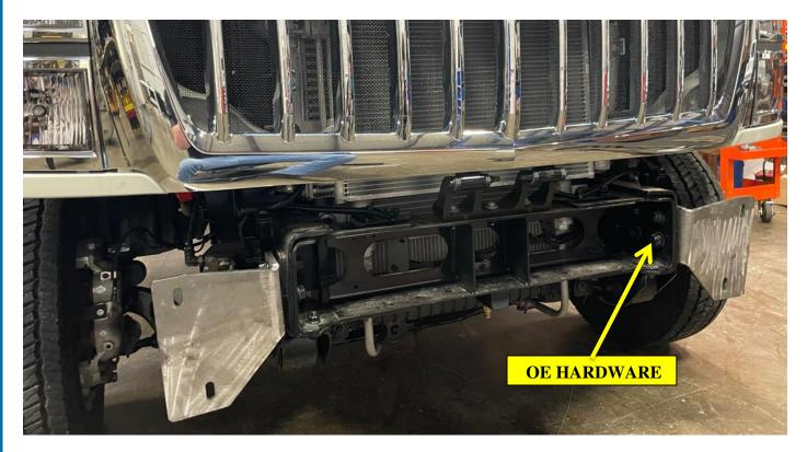
3. Using a hoist or a few friends, attach bumper to frame mounts using hardware kit #208. Start all bolts before aligning bumper. Align bumper a minimum of <sup>1</sup>/<sub>4</sub>" below plastic fascia. When truck flexes off-road, this distance allows your bumper and body to have clearance. Fully tighten bolts with <sup>3</sup>/<sub>4</sub>" socket. Fully tighten frame mount bolts as well at this time.
