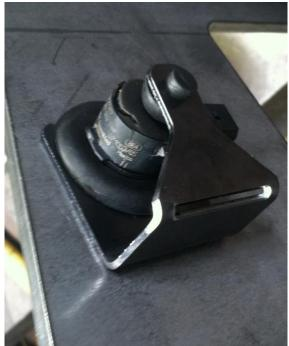
4. Using a 13mm socket, remove the upper OE bolt on the inside of the OE bumper as pictured below. Install left upper mount (*Item 2*) using M8 hardware supplied in hardware kit #229 with notched tab of upper mount on the OE bumper side. Ensure upper mount fits snug to top of OE bumper and curves away from the center of the truck. Repeat for other side.
