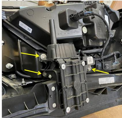
6. Using a torx 30 drive, remove four bolts holding OE fog lights in bumper. Carefully unplug fog lights from harness. Remove housing and set aside. (Both sides)
