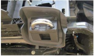
4. Using a 15mm socket, remove 2 bolts attaching OE tow hook to frame. Set tow hook aside (both sides). Keep the bolts and nut strips, they will be used again.
