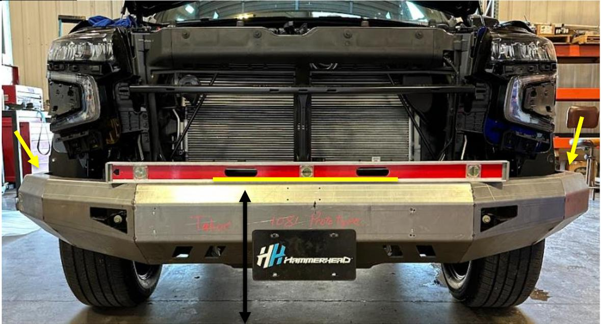
5. Next, remove the bumper and frame mounts. Place bumper and frame mounts on a carpeted surface or on a piece of cardboard.
