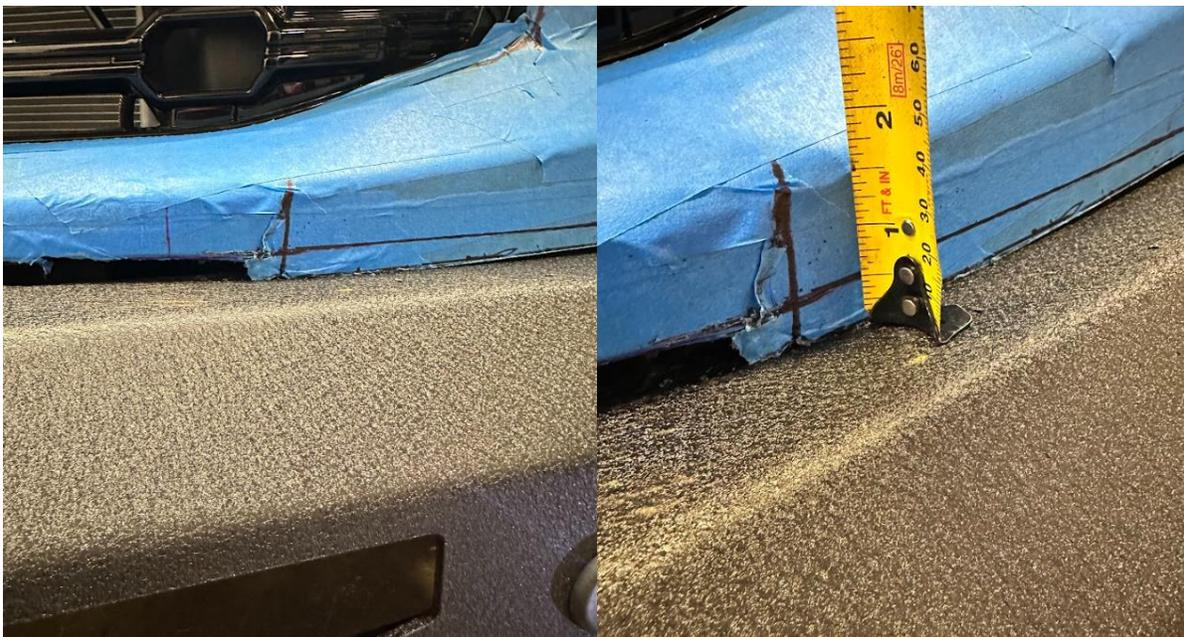
14. Before cutting, the bumper can be loosened and angled out of the way. Put on safety glasses, face shield, earplugs, and gloves. Using a cutoff wheel, oscillating multi tool, electric grinder, or air die grinder, cut the second cut line across the grille. Go slow and take your time.
