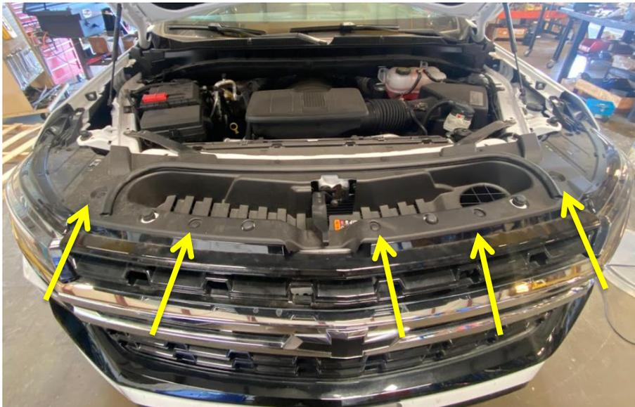
2. On each side of the vehicle, locate the (6) T15 screws (3 per side). This will give you access to the (6) 7mm bolts (3 per side) holding the fender onto the body. Remove these and set aside for reuse.
