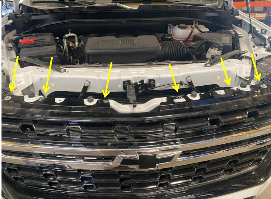
6. With the bumper removed, you can now remove the lower air guide. The lower air guide is held in place on the bottom with (4) plastic rivets. Using a trim removal tool remove the inner plug then the outer plug will pop out.
