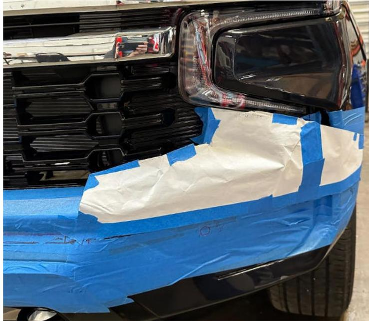
10. Put on safety glasses, face shield, earplugs, and gloves. Using a cutoff wheel, oscillating multi tool, electric grinder, or air die grinder, cut the 1<sup>st</sup> cut line across the grille. Go slow and take your time.
