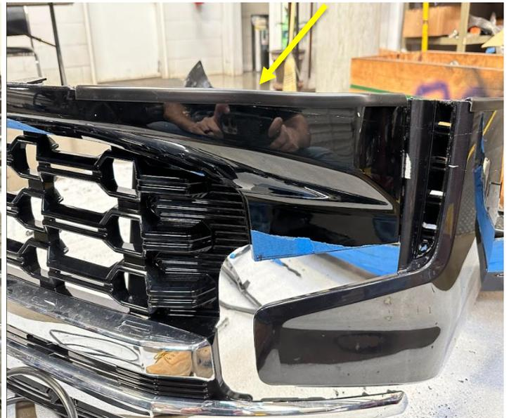
17. Next, start attaching the grille from the center and working your way out. This allows for the clips to line back up properly making sure the grille is on correctly. Work your way out to the fender flairs.
