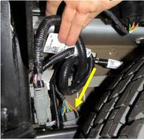
3. Using 10mm socket, remove bolt attaching wiring harness ground to truck. (located outside frame rail on left side)
