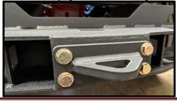
3. Using a hoist or a crane, loop a strap through the slots in the bumper as pictured below. Align bumper to be centered on vehicle and fully secure bumper to frame mount weldment using hardware from hardware kit #42. Use tow attachment and opening in bumper to help center. Using a 1/18" wrench and socket, fully tighten all hardware.
