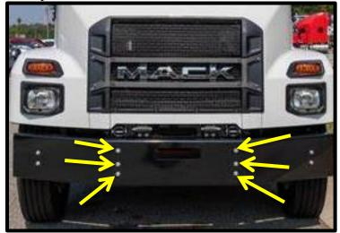
2. Using a 21mm socket, ratchet extension, 18mm wrench, and 24mm wrench, remove 3 OE bolts retaining OE bumper mount as shown below. Remove OE bumper mount and set aside. Set OE hardware aside to be re-used. Repeat for other side. (*Right side shown*)
