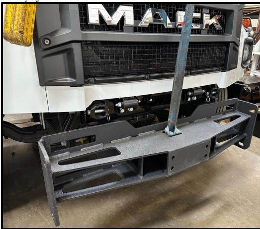
2. Using hardware from hardware kit #42, install tow attachment (*ITEM 3*) to front of frame mount weldment as shown below. Fully tighten all hardware using 1 1/8" socket and wrench.
