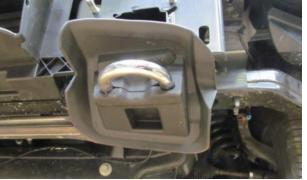
4. Using a 15mm socket, remove 2 bolts attaching OE tow hook to frame. Set tow hook aside (both sides). Keep the bolts and nut strips, they will be used again.
