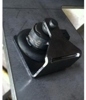
4. Using a 13mm socket, remove the upper OE bolt on the inside of the OE bumper as pictured below. Install left upper mount (*Item 2*) using M8 hardware supplied in hardware kit #229 with notched tab of upper mount on the OE bumper side. Ensure upper mount fits snug to top of OE bumper and curves away from the center of the truck. Repeat for other side.
