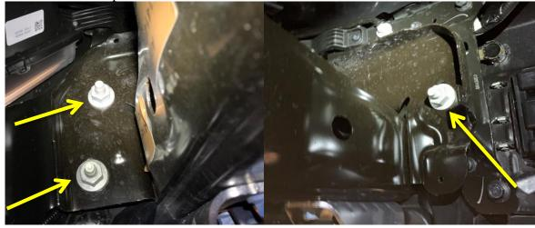
3. Remove OE tow hook shroud by pulling away from the truck. (Both sides)
