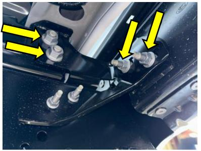
3. Using a 13mm socket, remove two bolts attaching bumper to receiver hitch. Bumper is now free to be removed. Set aside as it will not be reused.
