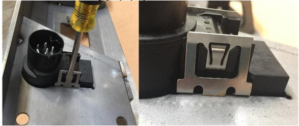
3. Install OE license plate lights into HH bumper as shown below. Note location of tabs and notches.
