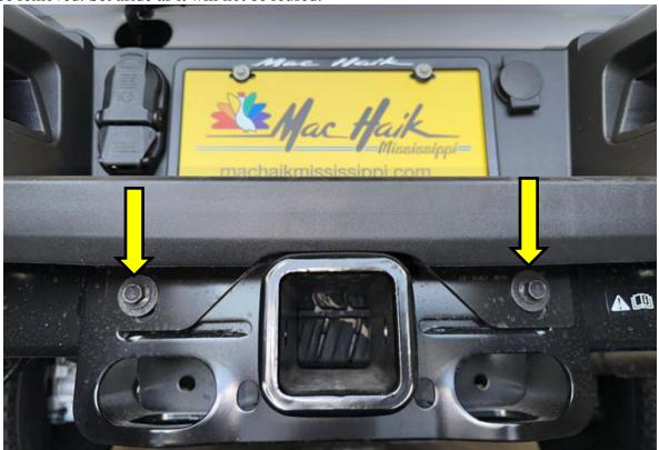
4. Using a 21mm socket and a 13mm socket, remove OE bumper frame mount from frame of truck. Repeat for other side.
