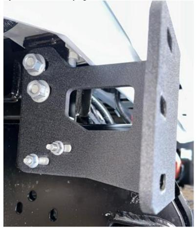
6. Using hardware kit # 53 and two weldnut tabs, attach bumper to HH frame mounts. Do not fully tighten.
