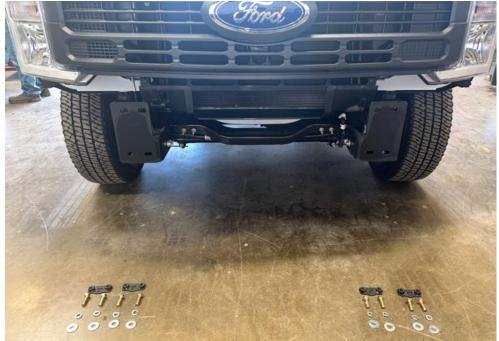
5. Using a hoist or a few friends, attach bumper to frame mounts using hardware kit #53 and weld nut tabs as shown below. Start all bolts before aligning bumper. Align bumper a minimum of ½" below plastic fascia. When truck flexes off-road, this distance allows your bumper and body to have clearance. Fully tighten bolts with ¾" socket. Fully tighten frame mount bolts as well at this time.
