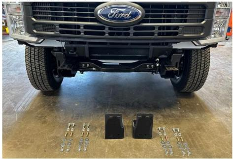
3. Install frame mounts on frame with hardware from kit #98. Insert bolts from the top. Use bolt strips removed in step 6 to attach HH mount on both sides of frame. Do not fully tighten.
