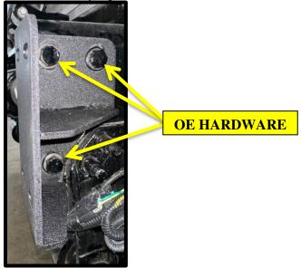
3. Layout hardware from hardware kit #62 as well as weld nut tabs from install kit. Using the help of a hoist or crane, secure bumper to left and right frame mount weldments. Ensure hood has enough clearance to open. Using a <sup>3</sup>/<sub>4</sub>" wrench or socket and tools from removal steps 2 and 3, fully tighten all hardware.
