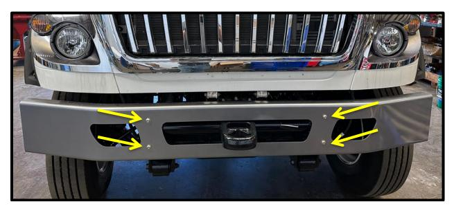
Using a 15/16" socket and 15/16" wrench, remove 2 bolts retaining OE bumper mount to frame. Remove and set aside. OE hardware will be re-used but OE bumper mount will not. Repeat for other side.
