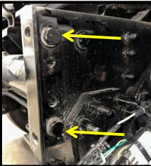
3. Using the same tools from the previous step, remove third OE bolt from frame. Set hardware aside to be re-used. Repeat for other side.
