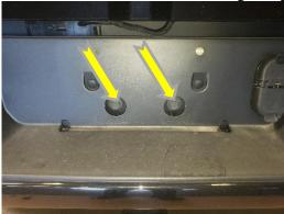
5. Remove the two nuts holding the bumper to the frame on both sides. You will use a 16mm socket.
