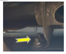
11. Align and level bumper with the truck. Tighten the center bolts with a 15mm socket and bumper mount bolts with a 3/4 wrench and socket. Install license plate mounting kit and license plate on bumper.
