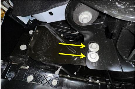
3. Using a trim tool or flathead screwdriver, remove trim piece from around tow hooks.
