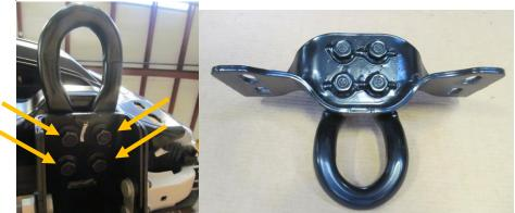
6. Using 18mm socket, remove two nuts attaching underrun bracket to frame. Set aside; it will not be reused. (both sides) Bolt strips and nuts will be reused.
