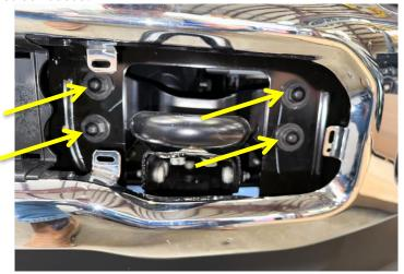
5. Using an 18mm socket, remove four bolts attaching tow hook to frame. Set aside; it will not be reused. (both sides)
