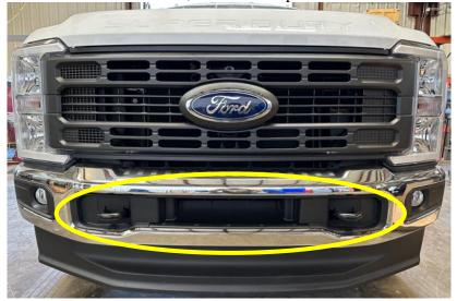
4. Using an 18mm socket, remove eight bolts attaching the bumper to the frame. Remove bumper and set aside. It will not be reused.
