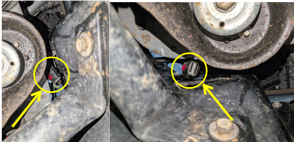
Figure 1: Depicted above is the passenger side wiring harness connection from below the truck oriented towards top of the vehicle.
