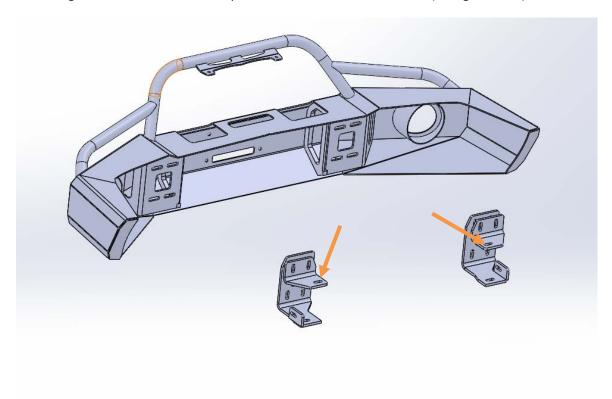
2. In this step you will use hardware from kit #4. Using two ½"-13 x 2.00" bolts, four ½" flat washers, two ½" lock washers, and two ½"-13 hex nuts attach Hammerhead lower mounts to OEM frame. (orange arrows) One bolt will go in the side of the frame and one will go through the bottom of the frame. (both sides)
