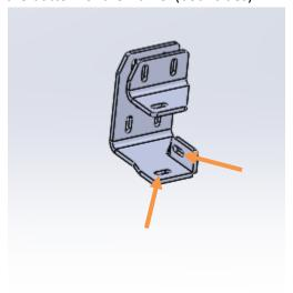
3. In this step you will use hardware from kit #1. Using eight ½"-13 x 2.00" bolts, sixteen ½" flat washers, eight ½" lock washers, and eight ½"-13 hex nuts attach Hammerhead bumper to Hammerhead frame mounts. (orange arrows) Align and tighten all hardware using a ¾" wrench and socket.
