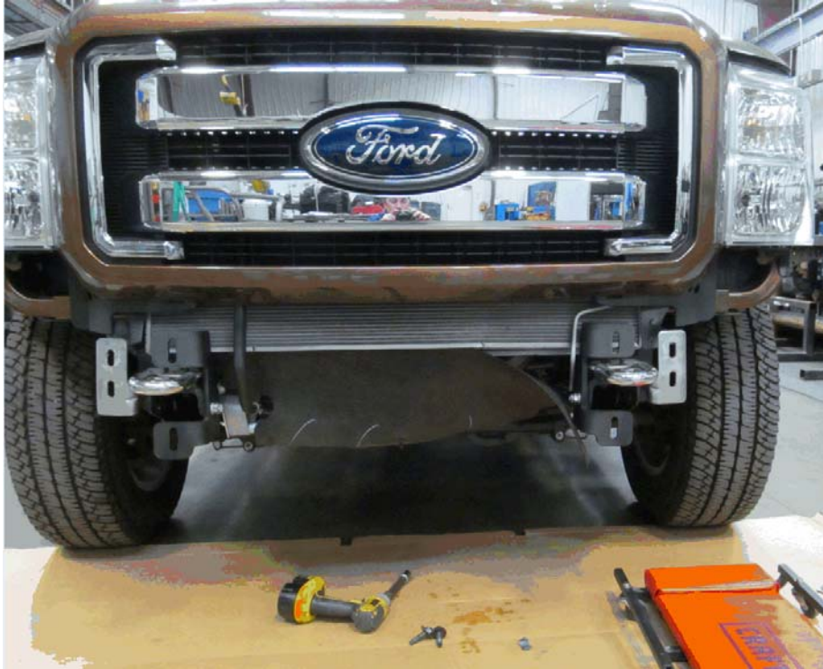
Front end with Hammerhead frame mounts installed
