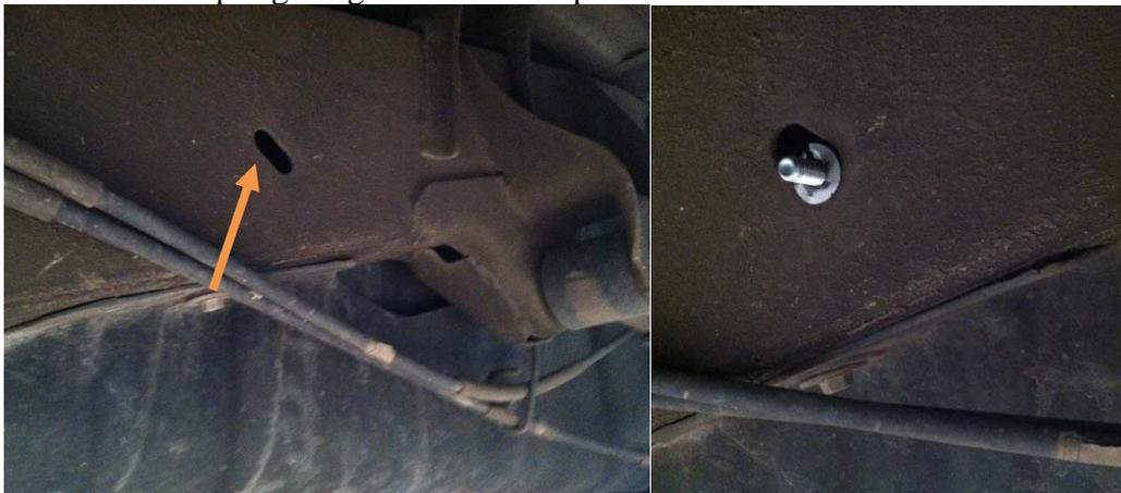
3. Have a good friend help you hold the running board's rear mount up to the bolt tab weldment you just installed. Using one 3/8" flat washer, one 3/8" lock washer, and one 3/8-16 nut, install the rear mount. Hand tighten.
