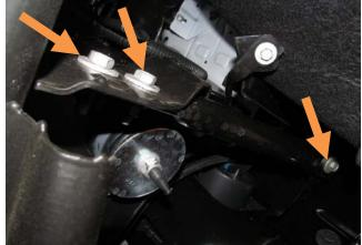
9. Remove OE bumper bolt with 18mm wrench. (both sides) Remove OE bumper and set aside.
