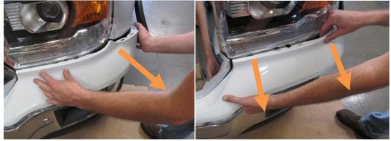
5. Release six tabs on center of plastic trim below the grill. Have a friend gently pull out on the plastic trim as you release the tabs behind the
