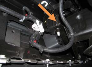
8. Remove three bolts from OE side bumper support (in front of tires) with 15mm socket. (both sides)
