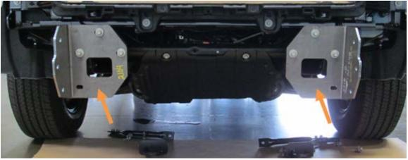
3. Install Hammerhead lower frame mounts (601-56-2155 and 601-56-2156) and loosely tighten. Use OE hardware for thru frame bolt and use two ½"-13 x 2" bolts, four flat washers, two lock washers and two nuts from Hardware kit #1 for the lower bolts. (orange arrows).
