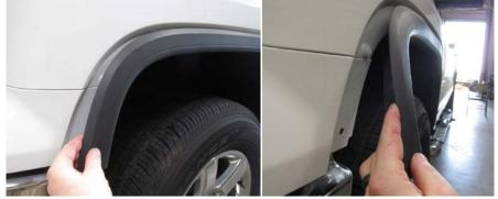
3. Remove screw holding on plastic trim piece with 7mm socket. (both sides)
