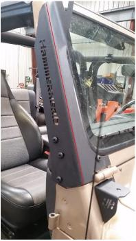
2. Install the opposite side the same way. Do not tighten bolts yet.
