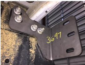
9. Using hardware kit # 53 and two weldnut tabs, attach bumper to HH frame mounts. Do not fully tighten.
