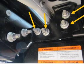
3. Using 13mm socket, remove two bolts attaching bumper to receiver hitch. Bumper is now ready to be removed. Set aside; it will not be reused.
