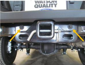
4. Remove license plate lights, trailer connector, sensors, sensor grommets, spare tire access lock, and wiring harnesses from bumper.
