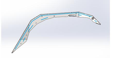
2. Place flare on the fender. The OE fender brace goes through the opening on the inside of the flare.
