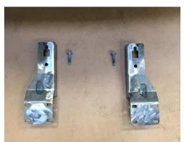
5. Slide mounts over rear OE frame bolt and install front bolt. Do not fully tighten.
