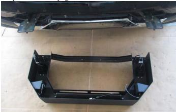
8. Route light wires down the uprights, and on top of the frame mounts into the truck's bumper. Secure them with zip ties.
