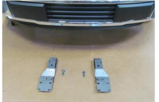
6. Slide mounts over rear OE frame bolt and install front bolt. Do not fully tighten.
