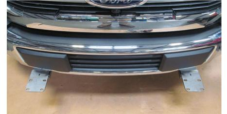
Lay down carpet or cardboard in front of truck. Layout Bull Bar as shown. Use hardware kit# 92 to attach bull bar to frame mounts. Use one 3/8"-16 bolt, one 3/8" lock washer, and one 3/8" flat washer per hole. Install all bolts. Using a 9/16" socket with 3" extension, tighten all bolts. Use torque values on page one.
