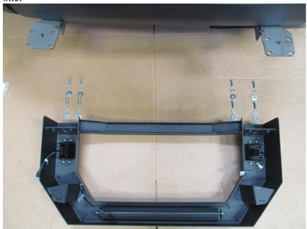
5. Have a friend help you align the Bull Bar. Push the top of the bull bar towards the truck. Using a 17mm socket, tighten the frame mount bolts at this time. Use torque values on page one.
