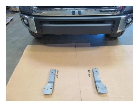
3. Install frame mounts where OE tow hooks were removed, using 17 mm OE bolts. Hand tighten the bolts.
