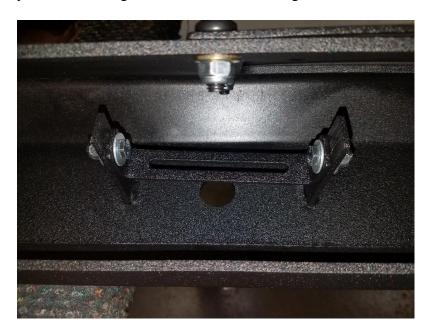
4. Bolt the rock rail to the jeep with the 3 body mount bolts you removed earlier as shown using the 18mm socket.
