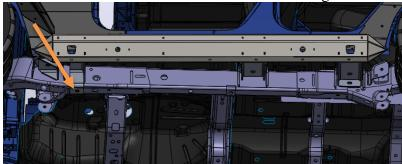
6. Install the provided 3.5in .5in bolt, nut, and washers from hardware kit #111 in the shown location. You will use the 3/4" socket and 3/4" wrench. Bolt will go all the way through the frame.
