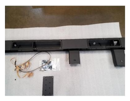
2. Using the 8mm bolts, washers and nuts from hardware kit #111 install the step plates as shown. You will use the Torx 40 and the 13mm wrench for this step. Make sure the step perforations are sticking up for grip.
