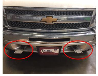
5. Lay down carpet or cardboard in front of truck. Lay Bull Bar as shown. Use hardware kit #92 to attach bull bar to frame mounts. Use one 3/8"-16 bolt, one 3/8" lock washer, and one 3/8" flat washer per hole. Install all bolts. Using a 9/16" socket with 3" extension, tighten all bolts. Use torque values on page one.
