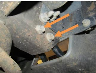
2. Using an 18mm socket and wrench, remove the tow hook bolts and the tow hooks. Set the hooks and OE bolts to the side, you will not use them again.
