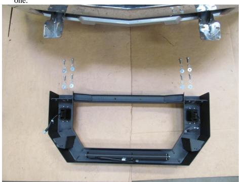
6. Have a friend help you align the Bull Bar. Push top of Bull Bar toward truck. Using a ¾" socket and wrench, tighten the frame mount bolts at this time. Use torque values on page one. Verify top of Bull Bar is level with ground.
