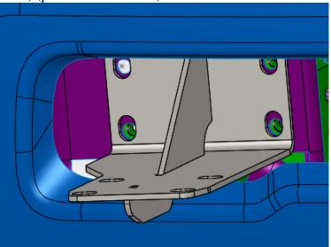
3. Lay down carpet or cardboard in front of truck. Lay Bull Bar as shown. Use hardware kit #92 to attach bull bar to frame mounts. Use one 3/8"-16 bolt, one 3/8" lock washer, and one 3/8" flat washer per hole. Install all bolts. Using a 9/16" socket with 3" extension, tighten all bolts. Use torque values on page one.
