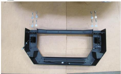
4. Have a friend help you align the Bull Bar. Push top of Bull Bar toward truck. Use torque values on page one. Verify top of Bull Bar is level with ground.
