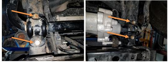
4. Place bumper on Jeep. Using 8 black <sup>1</sup>/<sub>2</sub>" carriage head bolts install the bumper. Bolts go through the shackle mounts, then the bumper. Use the provided <sup>1</sup>/<sub>2</sub>" nuts, washers, and lock washers to secure the bumper.
