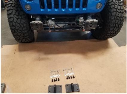
2. If you have the optional skit plat install that on the bumper now with the provided 3 hex head  $\frac{1}{2}$ " bolts. You will use a <sup>3</sup>/<sub>4</sub> wrench and socket.
