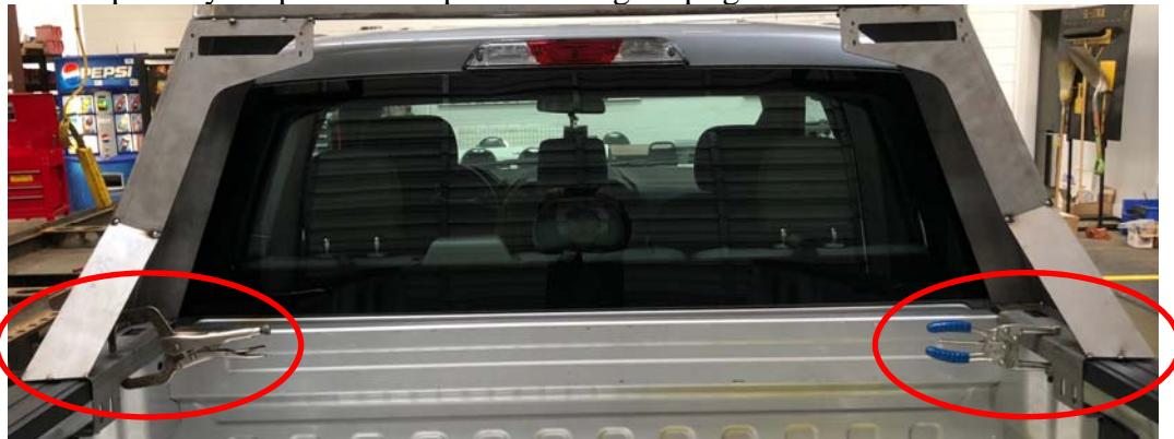
3. Using hardware from hardware kit #159, the nylon clamp block, and the nylon clamp spacer, secure the uprights to the side of the bed rail. Insert two Torx 40 bolts and two flat washers through the two slots on the side of the upright. Insert one  $\frac{1}{2}$ " hex bolt and one flat washer into the nut on the bottom of the upright. (See Pic) Do this for both sides. Use a Torx 40 bit and a  $\frac{3}{4}$ " socket or wrench to tighten the bolts
