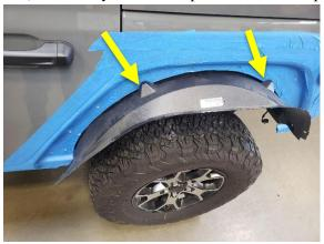
**c.** Cut the inner fender along the line you marked. A rotary tool is good for this job. TAKE YOUR TIME with the cut to produce a good visual result.
