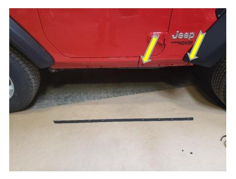
3. Place the trim piece on the Jeep. Using the Torx 30 socket install the two front replacement bolts. Use two 6mm bolts and two 6mm black washers as shown below.
