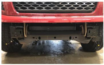
8. Remove the sensors, grommets, and sensor wiring harness from the OE bumper. **Be sure to note the position of the grommets, so that they can be installed in the correct locations on your new Hammerhead bumper.**
