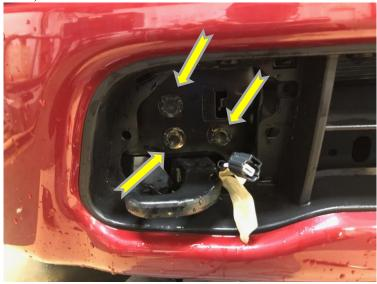
6. With the help of a friend, remove the OE Bumper by pulling it outwards away from the truck and set it aside.
