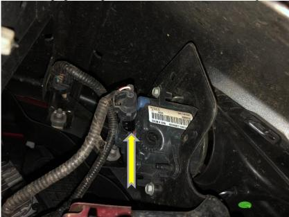
2. Disconnect the main sensor wiring harness. This connection is located next to the right side fog light.
