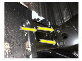
4. Remove the plastic covers around the tow hooks by pulling away from the front of the vehicle. Disconnect the sensor (if applicable). NOTE: When removing the covers be mindful of the sensor wiring harness so that you don't break the harness.
