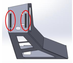
2. Using scissors, cut four 13.75" (350mm) length foam strips and apply two of them to the bottom of each upright (See Pic)
