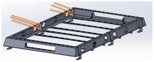
2. Using the torx 40 socket and the 13mm wrench install the remaining 14 bolts, nuts, and washers from hardware kit #112 to attach the cross braces on each side. (1 side shown below) Make sure to have the lip of the cross brace to the back of the roof rack. Square the roof rack and tighten all bolts.
