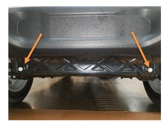
3. There is two nuts on the outside of the frame and the inside of the frame for a total of 8. Remove these with the 18mm socket.
