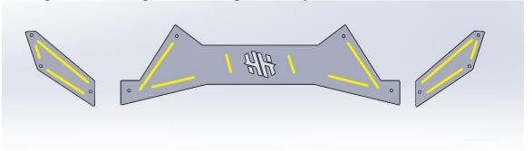
3. Install four  $\frac{1}{2}$ "-13 x 1.5" carriage head bolts in bumper with push nuts. Do this for both sides
