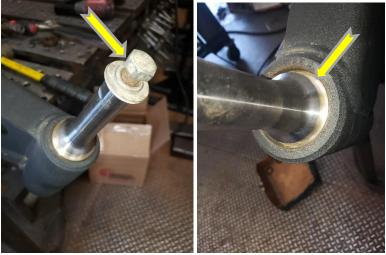
12. Press in the Aluminum O-ring insert next. You will use the Aluminum press in tool provided and a hammer to help you press it in.
