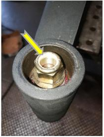
19. Install new cap into the top of the STC housing with the Aluminum press in tool. As shown below.
