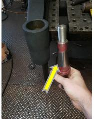
16. Place new roller bearing in the top as shown below. Make sure taper is pointing down.
