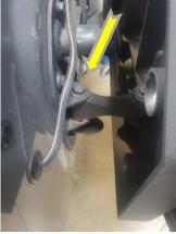
2. Remove the bolt holding the STC shaft into the rear bumper. Use a ¾" wrench.
