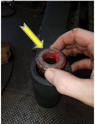
17. Place the provided new washer on top of the roller bearing as shown below.
