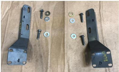
Install frame mounts onto the truck frame where the tow hooks were removed. On the rear hole, use one washer between the frame and the mount. Of the remaining washers, use 1 washer per bolt. Do NOT fully tighten.
